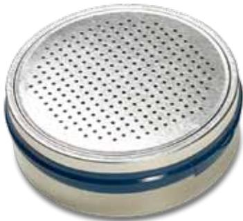
Radon Testing Corporation of America's short-term charcoal canister, \$47 for a two-pack
